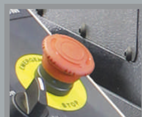
Emergency Stop button
